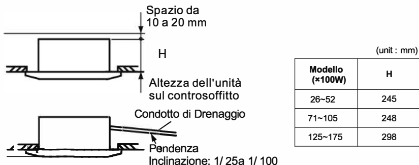
Fig. 3.2 Installation Location of Indoor Unit
